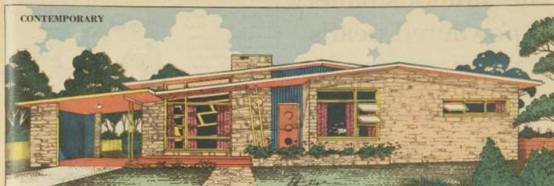
*PERSPECTIVE SKETCH (above) of contemporary design shows humped roof, sloping pergola, an attractive stone-faced chimney, and hopper windows. Carport, left.*
