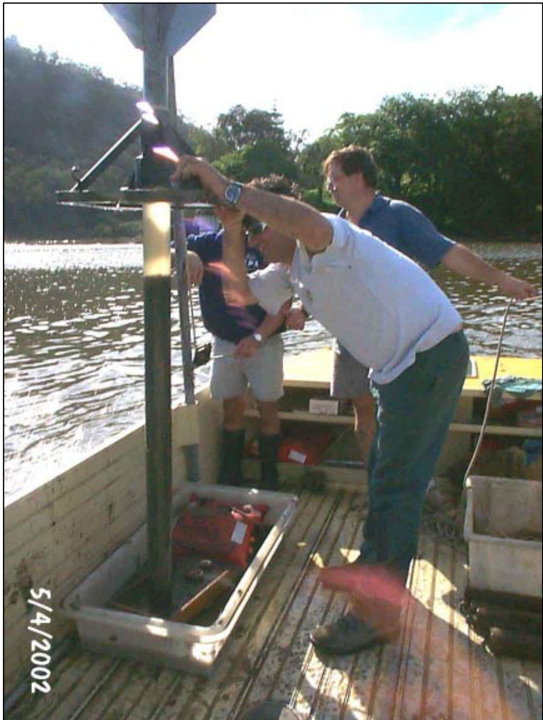
Figure 2. Gravity corer used in sampling program. Polycarbonate core barrel contains 1.3m long intact sample of estuarine bed.
