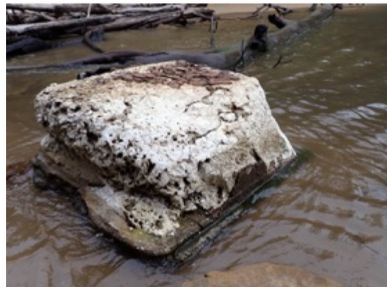
Timber logs from the bushfires washed into the Hawkesbury by floodwaters and concrete covered polystyrene pontoons decaying in the water
