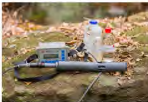
Figure 5.3: Sampling equipment used to measure water quality parameters. Sample are collected in bottles labelled with unique sample ID numbers.
