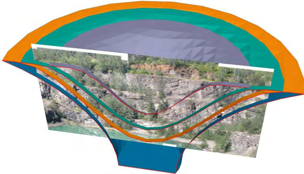
**Photo G3:** Face view illustration of eastern face in relation to “trumpet” shape of eastern diatreme body
