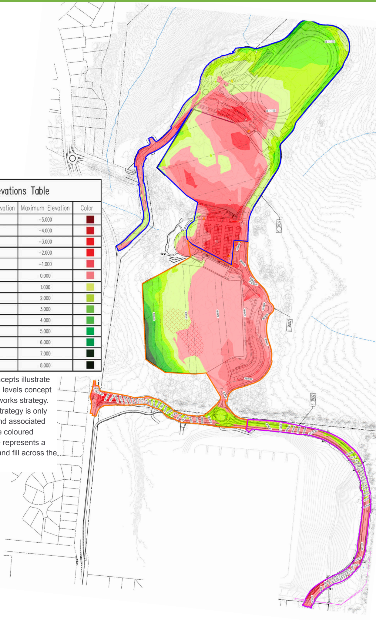
Figure 4.6 - Cut & Fill (Source: TTW)
