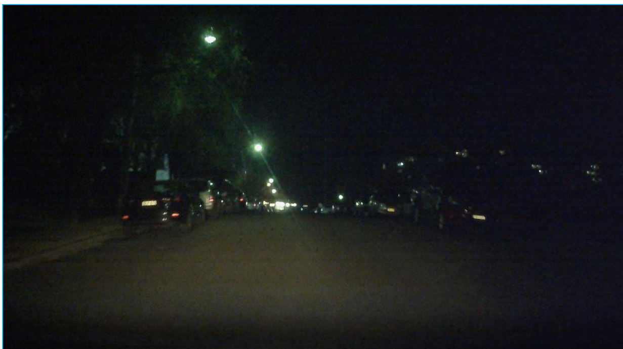
Figure 2-13: Trees obstruct lighting of street on Ashley Street
