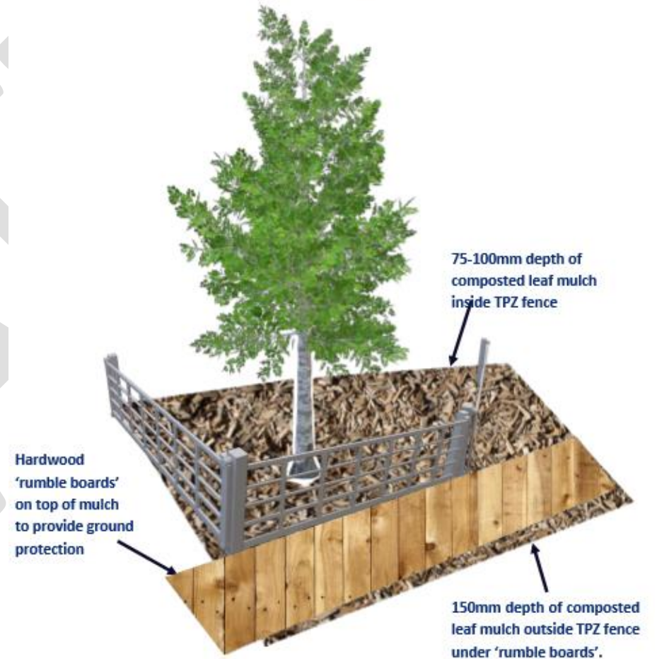
Ground protection: Access road within TPZ- Figure 2.
