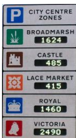
Figure C 16: Space counting VMS (Nottingham UK)
