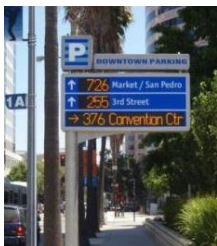
Figure C 15: Variable message sign (San Diego US)
