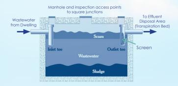
Bacteria in the septic tank break down the solid matter in the sludge and scum layers. Material that cannot be fully broken down gradually builds up in the tank and must be pumped out by a licenced contractor periodically.
