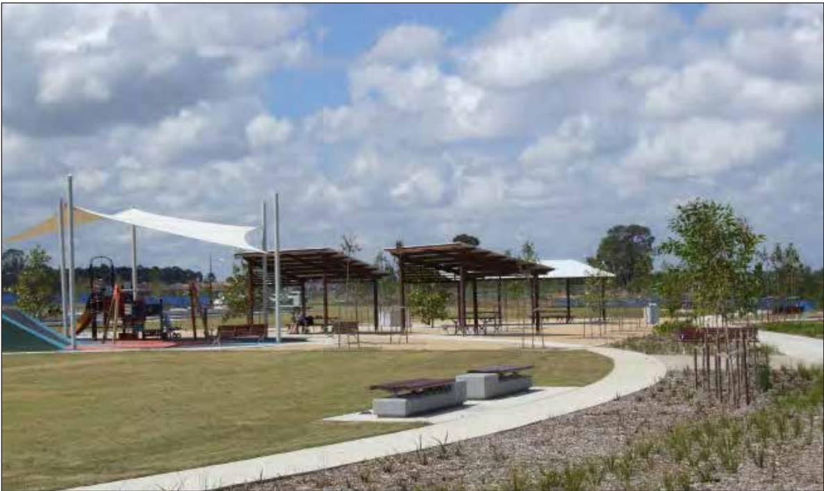
The use of boundary paths as management edges ensures that there is a clear definition of lawn area and provides an efficient and cost-effective mowing area.
