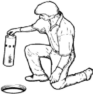
3. Check the absorption trench area is not soggy, doesn't smell and doesn't have prolific grass growth.
