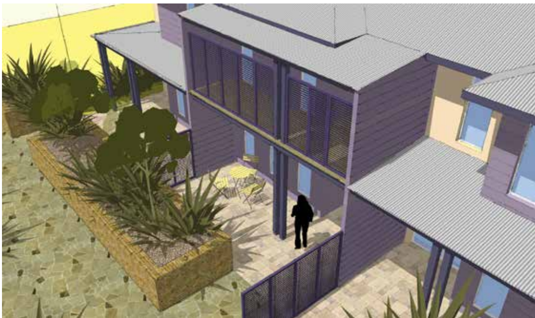
Figure 3.2(p): Fixed screens and communal planters provide privacy for ground level open spaces and rooms but allow casual surveillance of common areas from each dwelling. Adjustable screens on balconies provide for microclimate control. (E)
