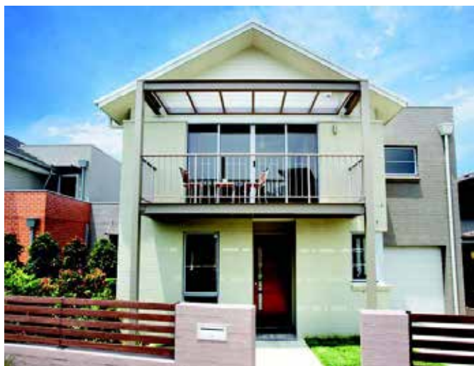
Figure 3.1(g): The main entry should be clearly visible from the street and sheltered from the weather, and the garages set back from the front facade. (E)
