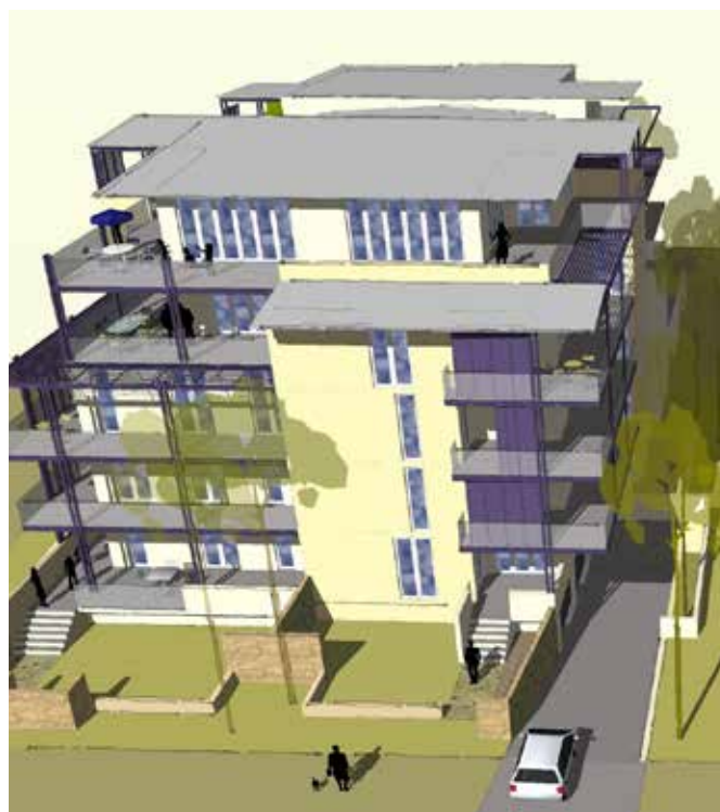
Figure 3.4(e): Building Height. (I) Height controls are based on a typical residential floor to floor height of 3 metres, with a 1.5 metre allowance for roof articulation and a 1 metre basement projection.
