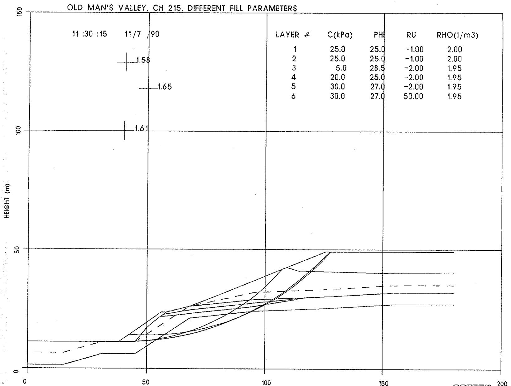
CH215G      SCALE 1: 1000. - SLOPE FLATTENED AT THE TOE 1(V):1.5(H),
