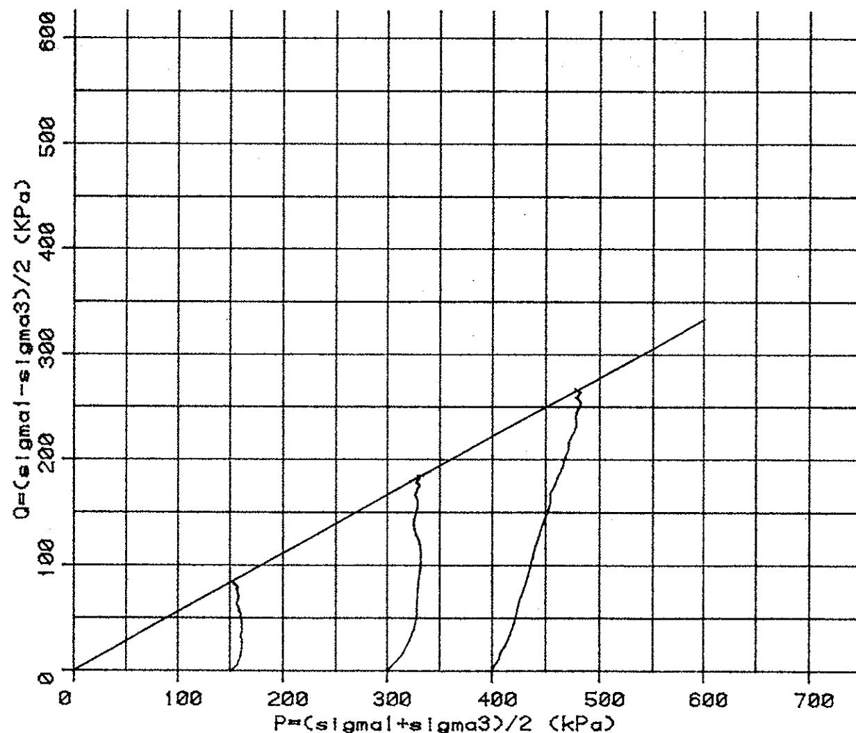
TYPE OF TEST : CONSOLIDATED UNDRAINED WITH PORE PRESSURE MEASUREMENT
