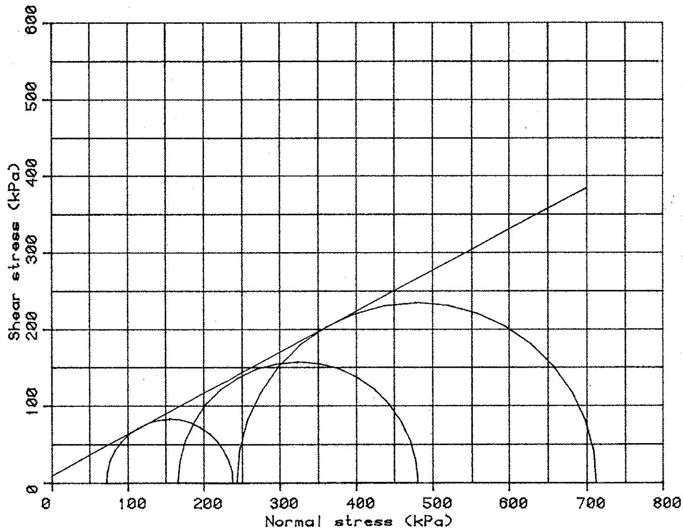
TYPE OF TEST : CONSOLIDATED UNDRAINED WITH PORE PRESSURE MEASUREMENT
