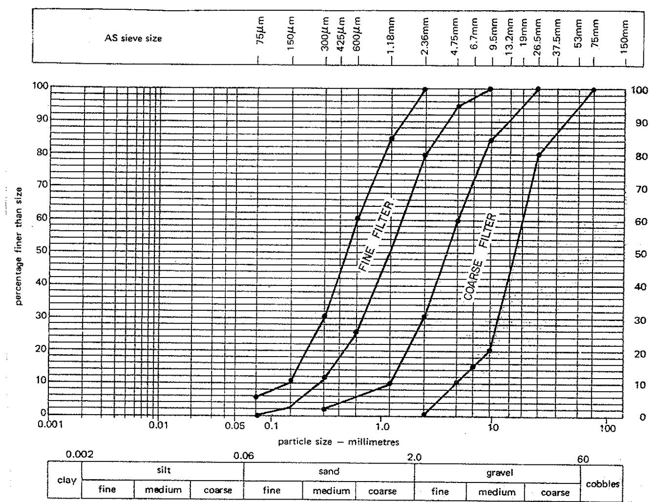
Graded filters, sand blanket material and gravel for geofabric drains shall conform to the requirements for concrete aggregate AS2758.1 except that grading shall be as shown above.
