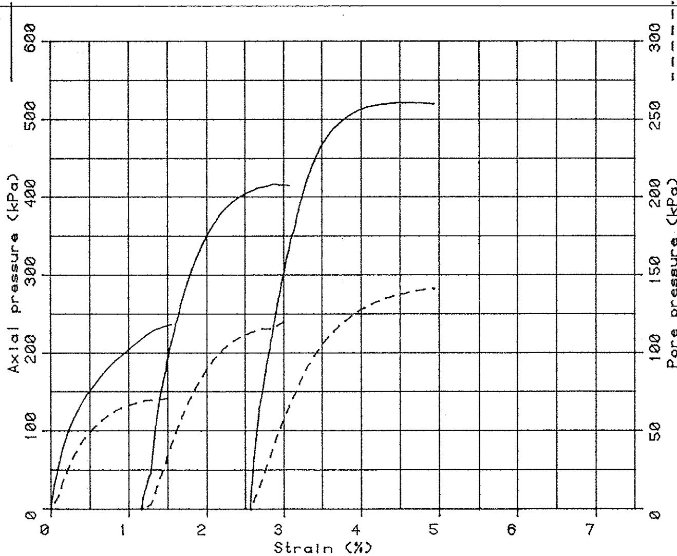
TYPE OF TEST : CONSOLIDATED UNDRAINED WITH PORE PRESSURE MEASUREMENT
