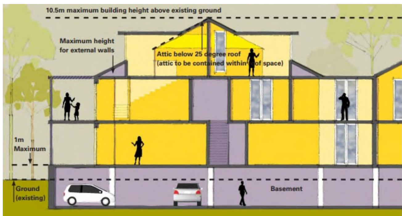
Figure 3.2-e: Building Height Controls - residential flat building of 2 storeys + attic. (I) Height controls are based on a typical residential floor to floor height of 3 metres, with a 3.5 metre allowance for roof articulation and a 1 metre basement projection.
