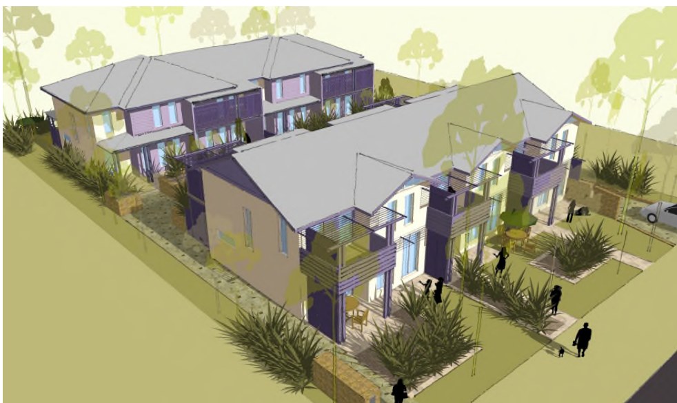
Figure 3.2-a: Town houses with basement parking are the most effective form of attached or multi dwelling housing. Positive responses to desired future character include deep soil landscaping along all site boundaries, dwellings that address the street or a central walkway, and that are not oriented towards neighbouring properties, and car parking that is concealed below ground level. (1)
