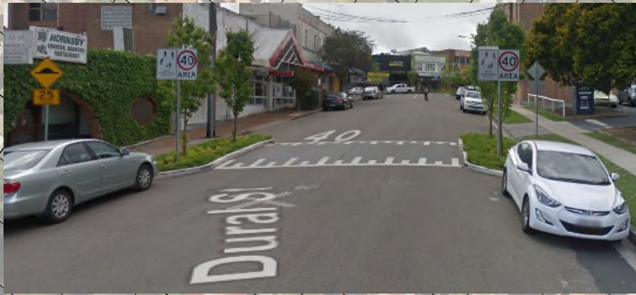
TYPICAL SPEED HUMP AND BLISTER ISLAND
