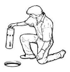
3. Check the absorption trench area is not soggy, doesn't smell and doesn't have prolific grass growth.
