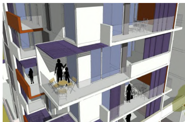
Figure 3.5-h : L-shaped balconies and terraces accommodate a number of activities, and adjustable screens provide shade, privacy and enclosure for outdoor rooms.(E)
