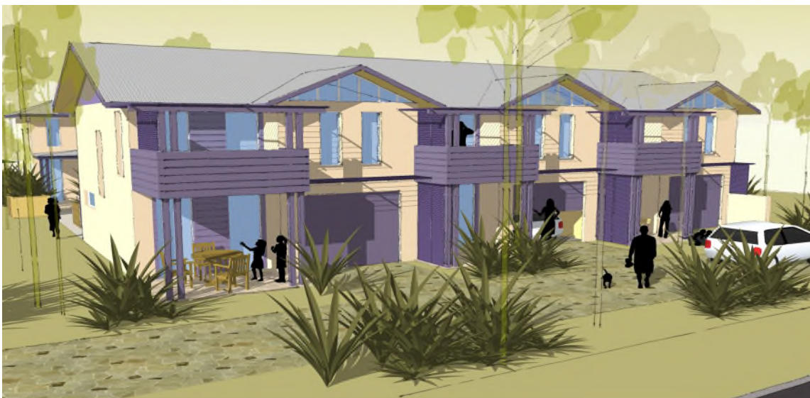
Figure 3.2-c: Town houses with ground level parking potentially provide for lower site yields and are not the preferred form for attached or multi dwelling housing. However where this built form is proposed, positive responses to desired future character include driveways that are flanked by landscaping, visible entrances to every dwelling and facades not dominated by garages. (I)
