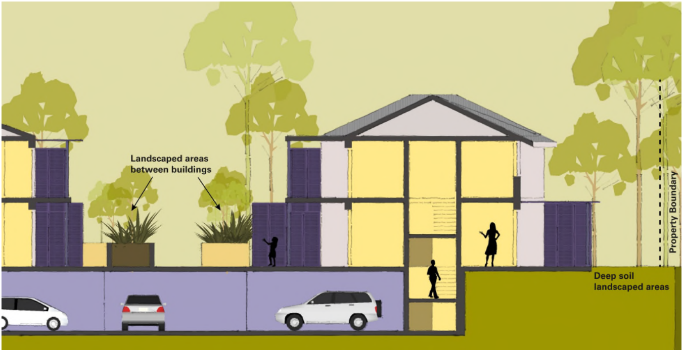
Figure 3.2-k: Landscaped areas for town house developments: deep soil adjacent to the property boundary and landscape planters between townhouses above basements. (l)
