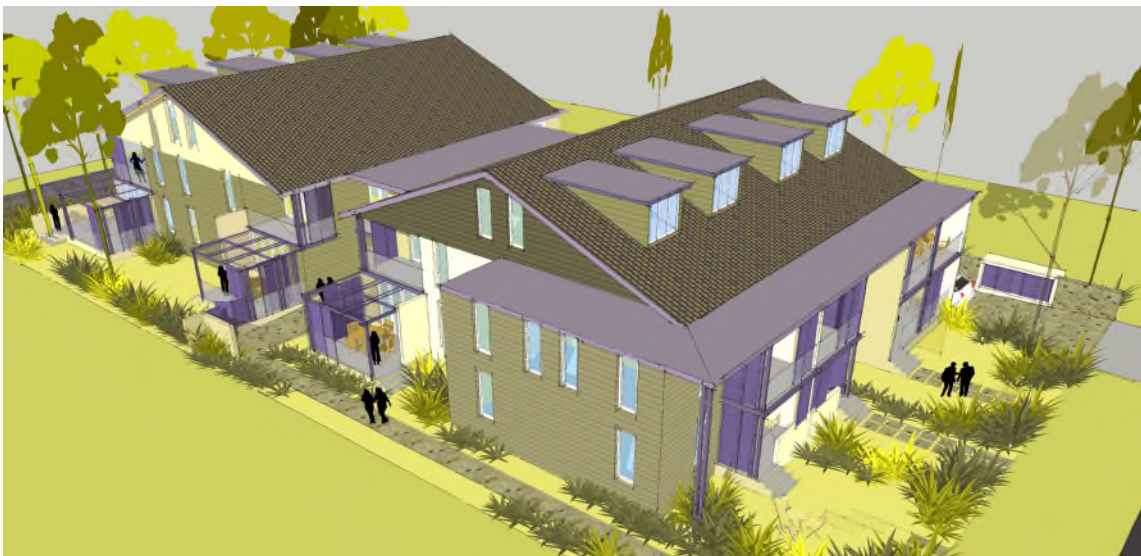
Figure 3.2-c: Town houses with ground level parking potentially provide for lower site yields and are not the preferred form for attached or multi dwelling housing. However where this built form is proposed, positive responses to desired future character include driveways that are flanked by landscaping, visible entrances to every dwelling and facades not dominated by garages. (I)
