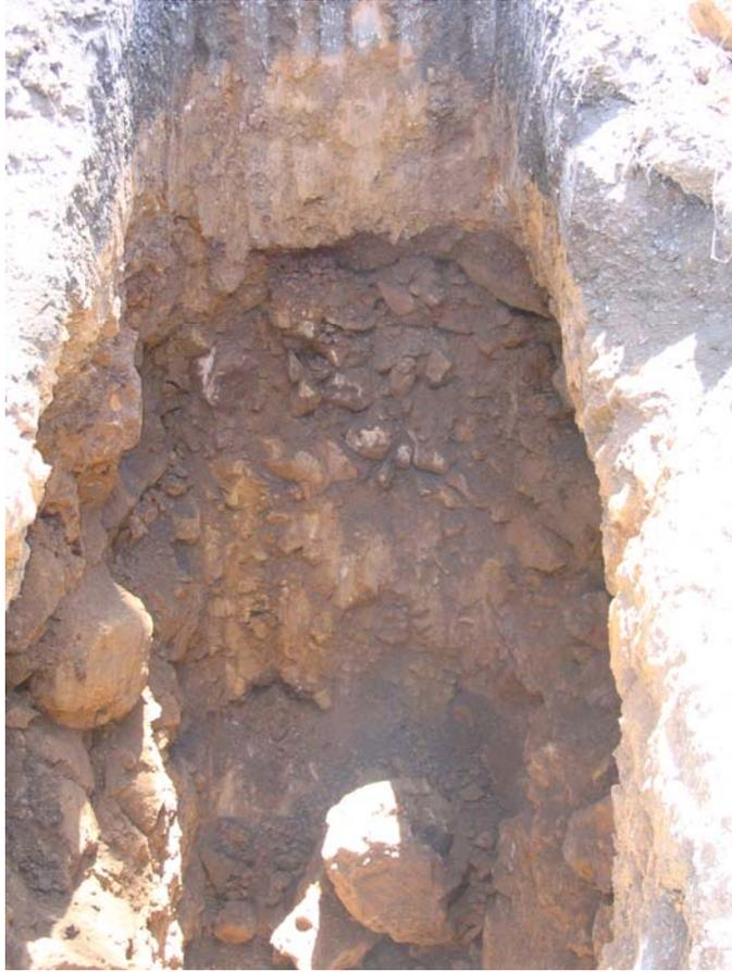
**TP3: Pit – note sidewalls collapsing**
