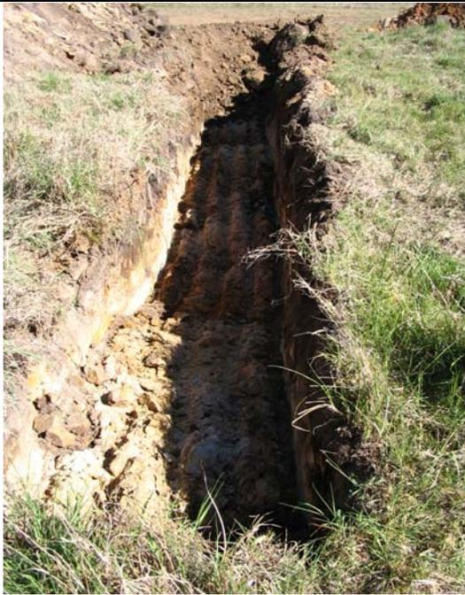
Longitudinal photo of pit; residual sandstone below topsoil in foreground (east); fill below topsoil in background (west).
