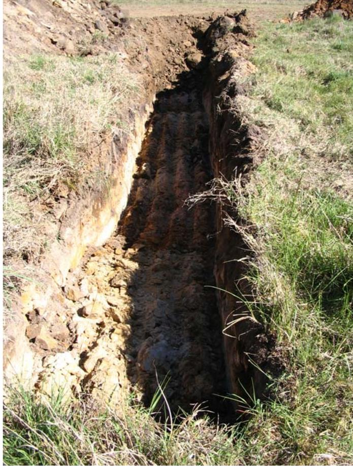
**TP11:** Trench showing sandstone at surface in foreground and fill at surface at opposite end of pit.
