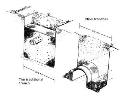
The failure of the trench is a common cause of problems with onsite sewage management systems. Trenches usually fail if the holes in the pipes that run through the trenches get blocked up, or if the effluent is unable to evaporate or drain away. You can tell if the trench has failed because the area will be soggy, smelly and covered with profuse grass growth.
