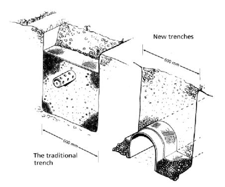
The failure of the trench is a common cause of problems with onsite sewage management systems. Trenches usually fail if the holes in the pipes that run through the trenches get blocked up or if the effluent is unable to evaporate or drain away. You can tell if the trench has failed because the area will be soggy, smelly and covered with profuse grass growth.
