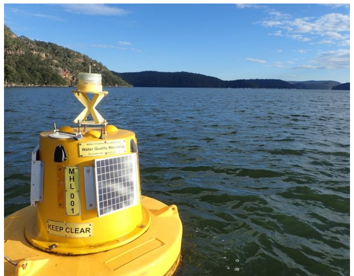
Figure 4.1: Remote water quality monitoring buoy at Gunya Point on the Hawkesbury River. The buoy houses a probe that measures several water quality parameters.
