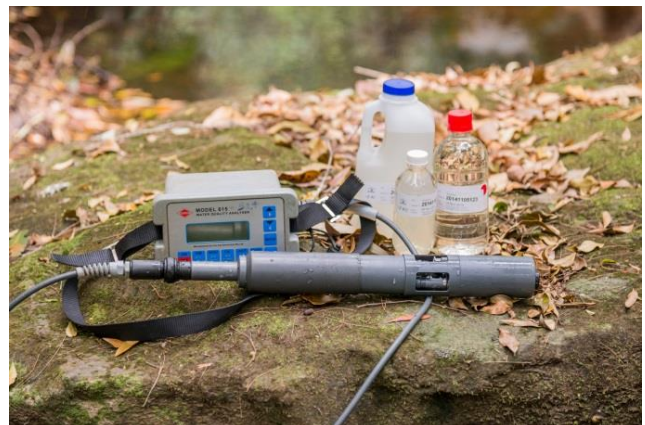
Figure 5.3: Sampling equipment used to measure water quality parameters. Sample are collected in bottles labelled with unique sample ID numbers.
