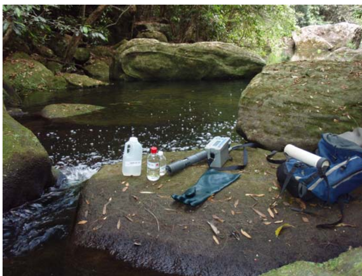
Photo 9. Equipment used for collecting water samples and recording in-situ water quality information
