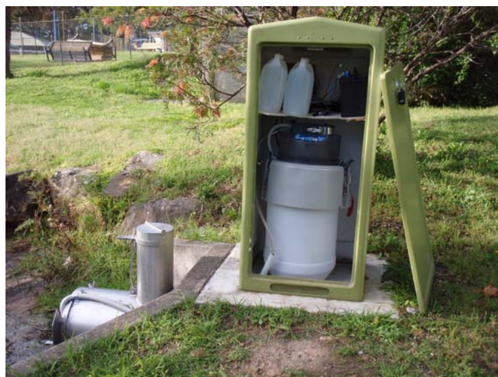
Photo 7. Site 148. Autosampler set up in Hornsby Park near a stormwater outlet to collect representative samples of running off Pacific Highway during storms.
