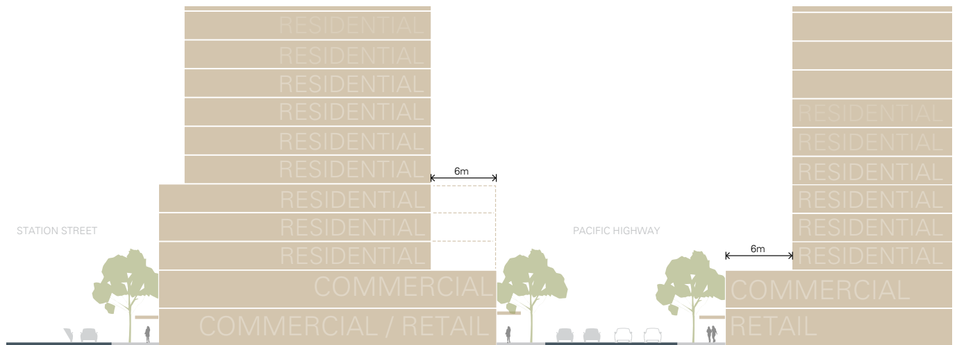
Figure 4.5(p): Upper level setbacks to Peats Ferry Road. (C)
