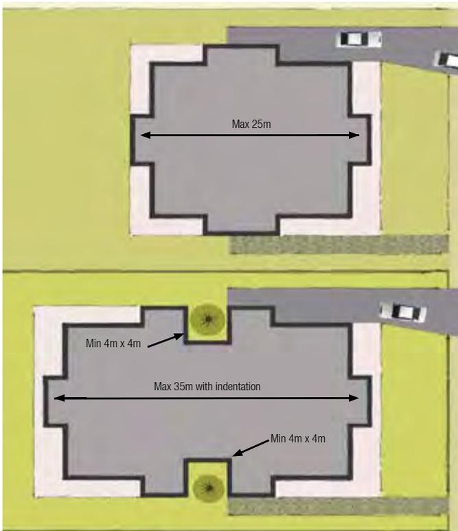
Figure 3.4(f): Building floorplates should be limited in width and depth.(E)
