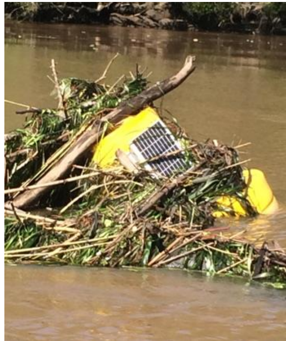
Figure 12 Loughtondale monitoring station buoy half submerged as a result of vegetation debris being collected on the mooring
