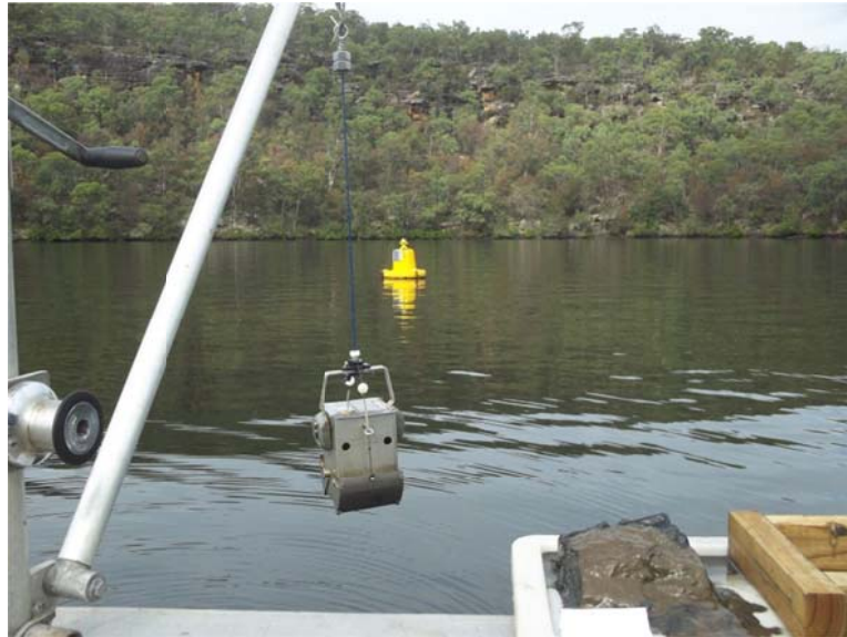
Plate 1 Sediment Grab in Operation at Berowra Creek (Location H7)
