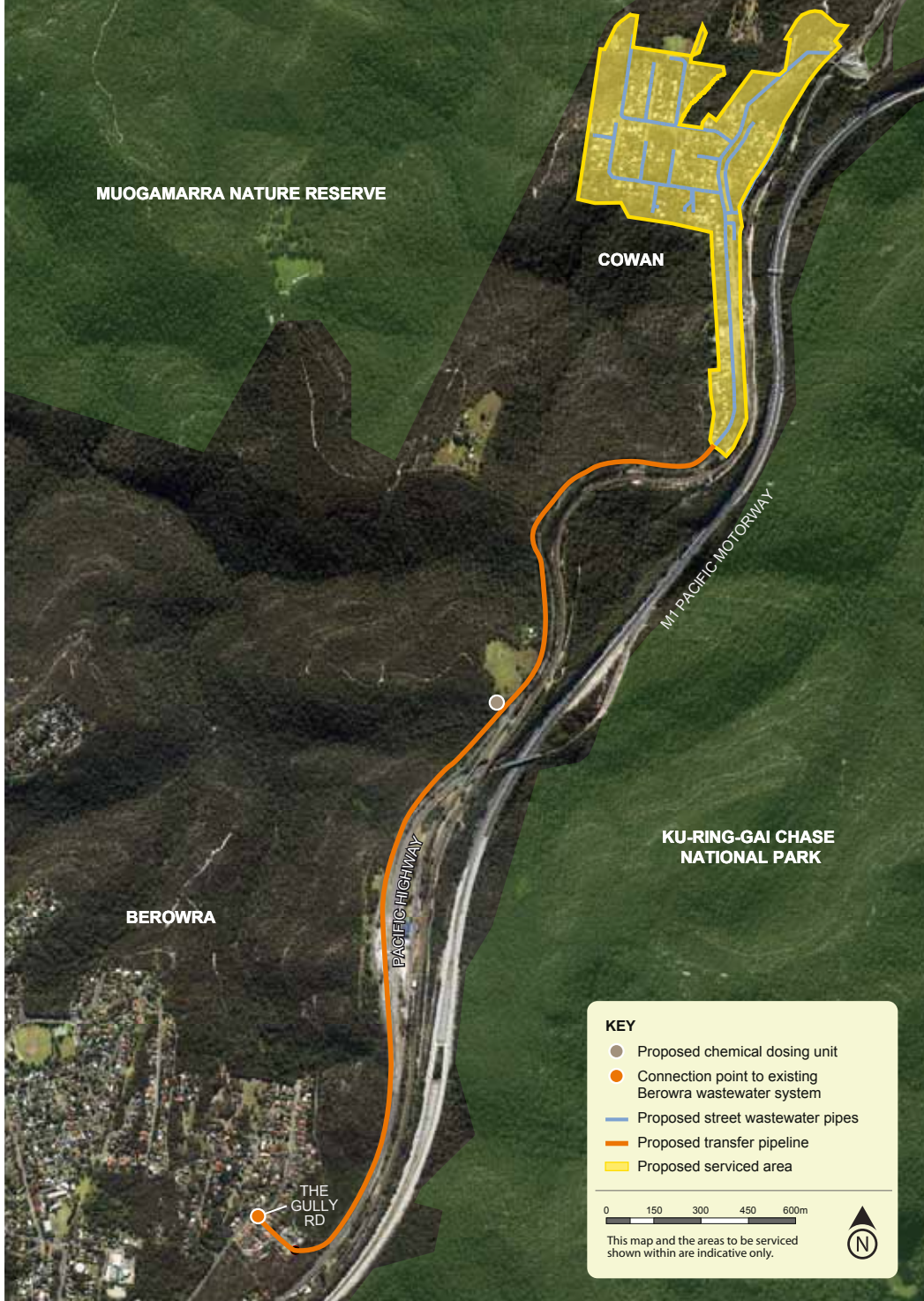
Figure 1 Scheme area map showing transfer pipeline
